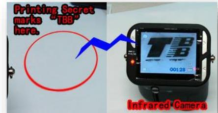
Invisible Code is microword and printed by invisible material
